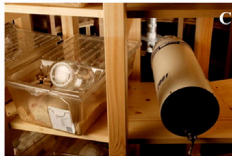
Fig. 1. RI study on 1.8 GHz base station RFR: exposure system. The rat cages were located in wooden circular-shaped devices, as in a sort of condominium. Each single exposure device served at least 400 rats (A). The exposure rooms were totally shielded in order to minimize the effect of field non-uniformity due to reflection and consequent interference caused by the walls (B). Detail of the RFR feedback probe used to measure the field (TESY2001 field sensor) and of the animal cage with methacrylate markers, cover and mangers (C).
