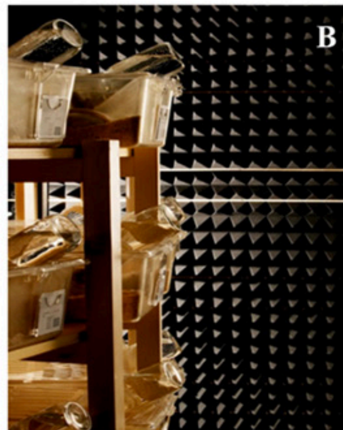
Fig. 1. RI study on 1.8 GHz base station RFR: exposure system. The rat cages were located in wooden circular-shaped devices, as in a sort of condominium. Each single exposure device served at least 400 rats (A). The exposure rooms were totally shielded in order to minimize the effect of field non-uniformity due to reflection and consequent interference caused by the walls (B). Detail of the RFR feedback probe used to measure the field (TESY2001 field sensor) and of the animal cage with methacrylate markers, cover and mangers (C).
